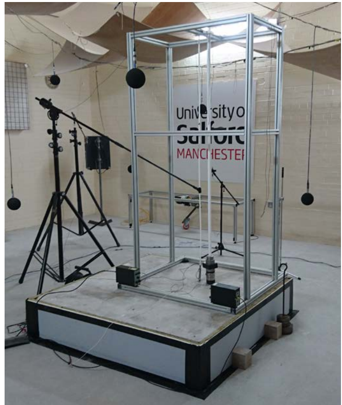
Figure 6: Drop test assembly on the bare concrete floor in the reverberation chamber
