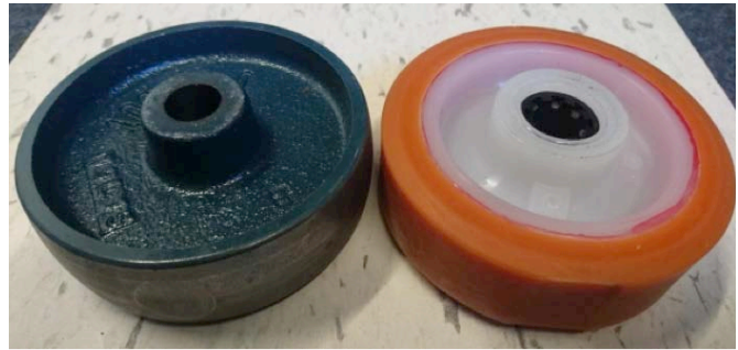
Figure 9: Steel and Polyurethane
